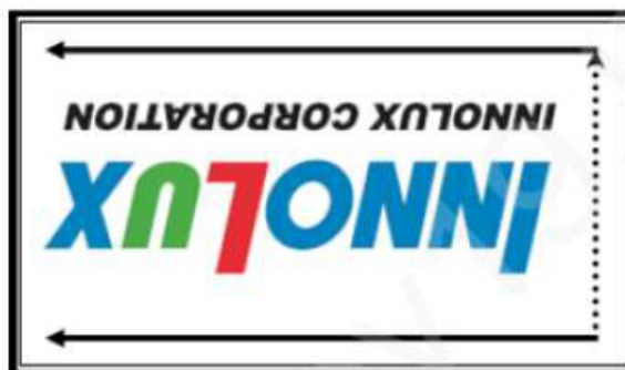
Fig. 2 Reverse scan (PCBA on the bottom side) ( pin 17, REV_SCAN = High )
